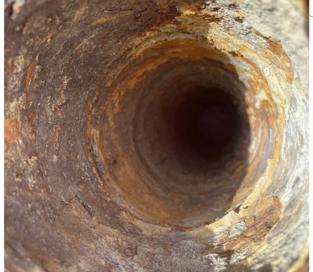
Corrosion from Positive Pressure System
