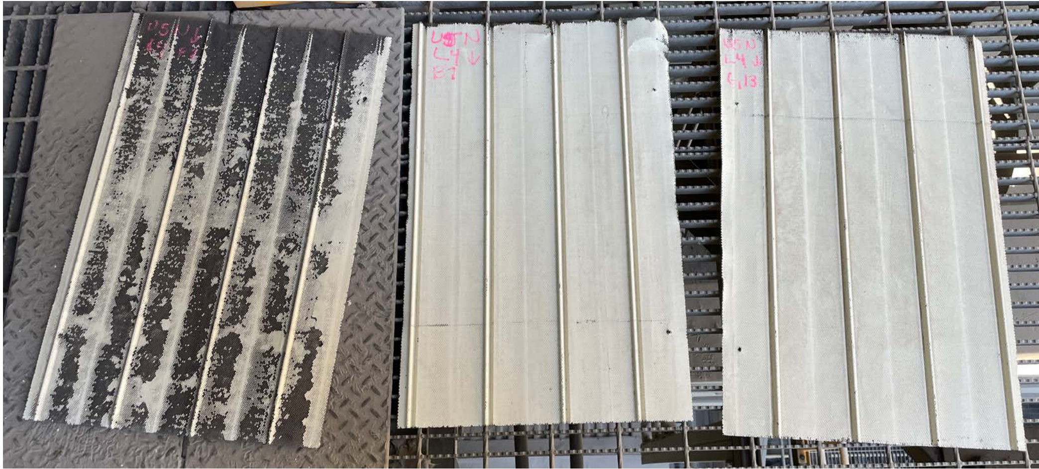
Unit 5 – Uneven Corrosion
