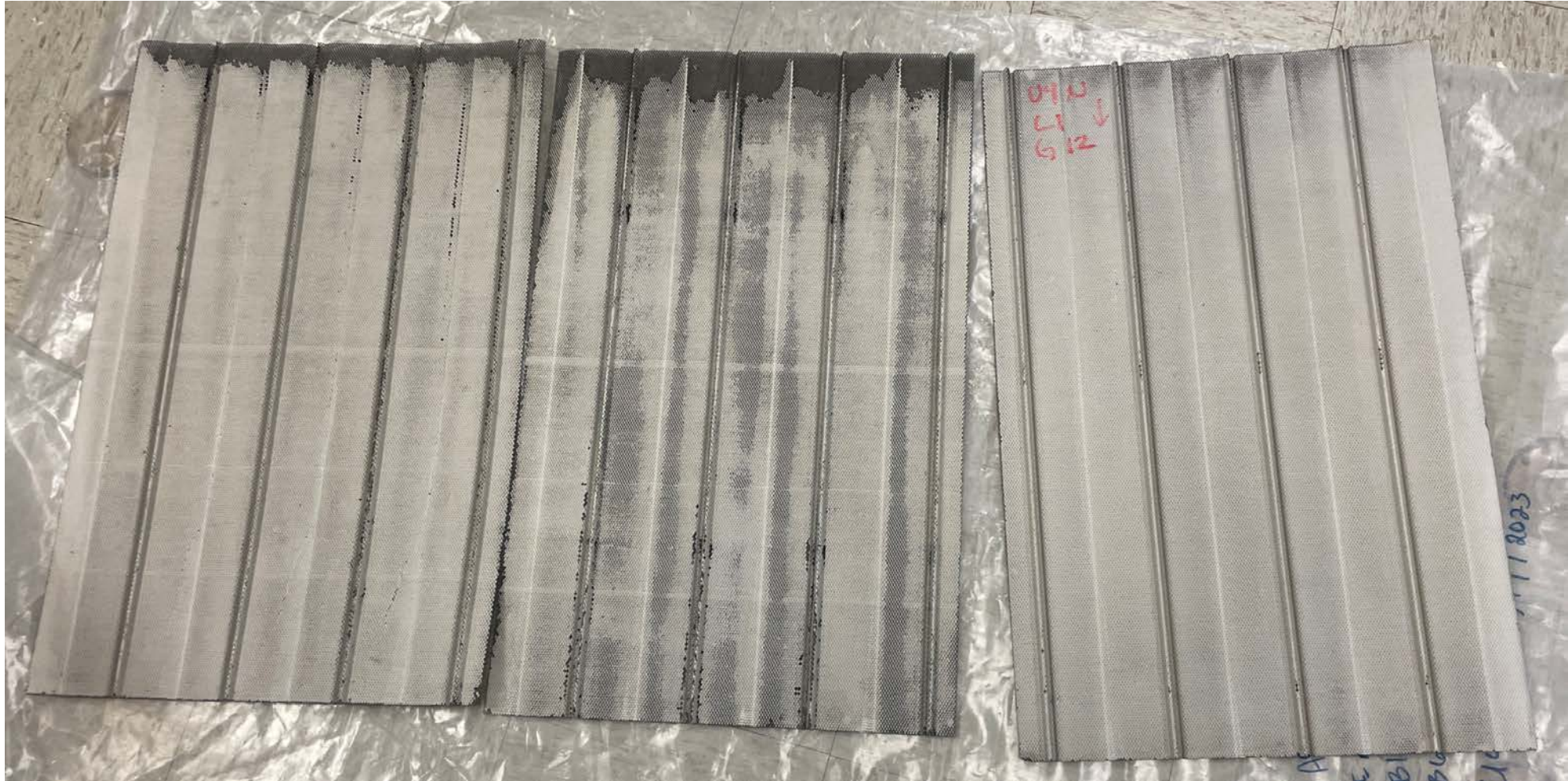
Unit 4 – Uneven Corrosion
